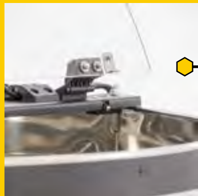
Safety lock - when the lid is opened, the basket is stopped
