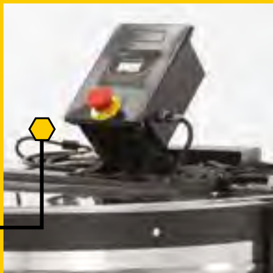
The controller has two manual programs and nine predefined automatic cycles. The controller also has one automatic program with the possibility of leading your own settings
